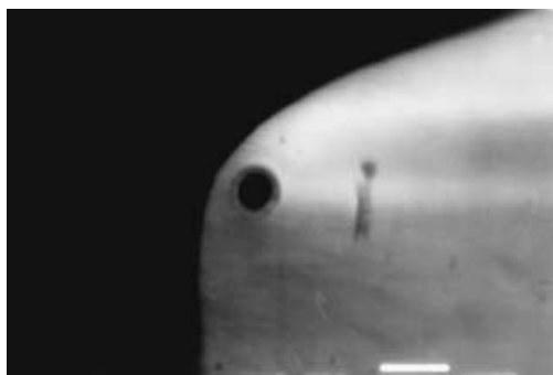
Figure 3. An SEM image of the pipet used in the experiments. Scale bar = 1 \mu\text{m} .
